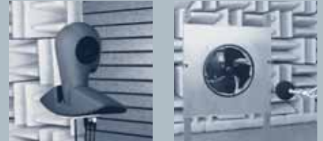
Room for precision noise measuring
